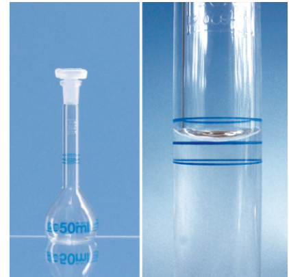
Measuring flasks with 3 marks. The 3 mark test plunger is used to check the function of a dispenser. The middle mark corresponds to the nominal volume, the upper and lower marks to the error limits
