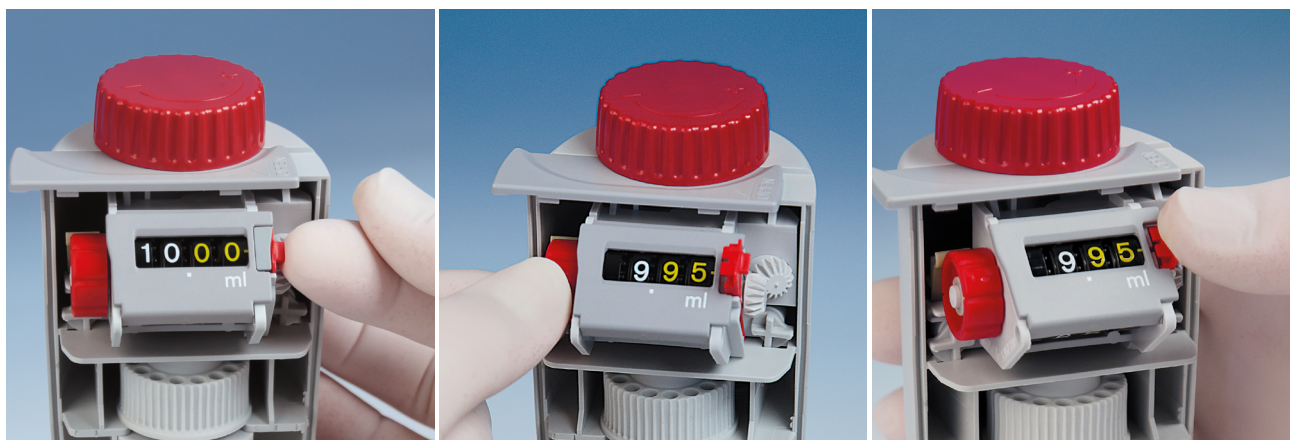
Adjusting a Dispensette S Digital – the volume displayed is adjusted to the actual measured volume.
